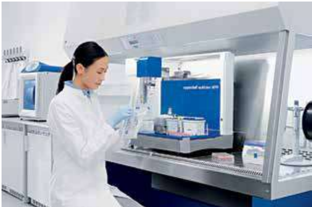
5070f integrated in laminar flow cell bench. The built-in light barrier beam monitors that the sash is closed for safe operation.
