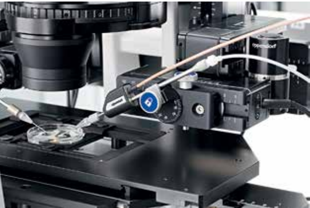
Eppendorf PiezoXpert actuator mounted onto TransferMan 4r
