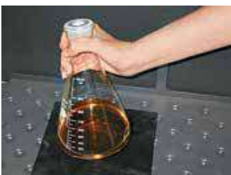
Sticky Pad (shown) and sticky tape replace clamps for speeds up to 250 rpm. Sticky Pad requires an anodized aluminum surface. (Not for use in water bath shakers)
