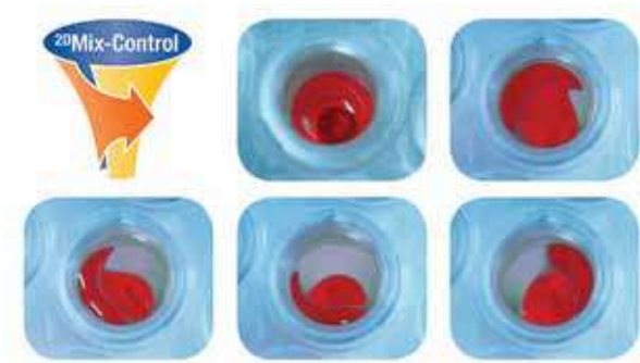
Time-lapse photography of controlled mixing with MixMate. The unique 2D Mix-Control technology mixes liquids in a very controlled, circular movement. The lack of chaotic splashing enables mixing without lid wetting or cross contamination.
