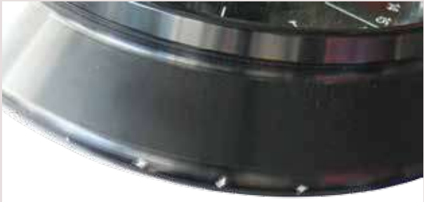
Rotor with internal “pitting corrosion”
