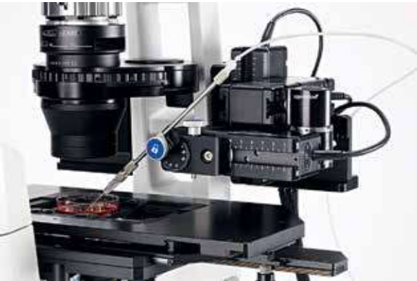
InjectMan 4 micromanipulator mounted for axial injection
