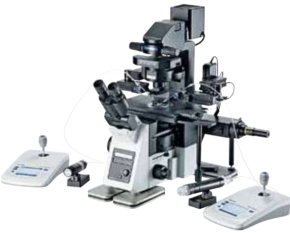
Workstation for cell transfer - TransferMan 4m mounted on Olympus® IX73
