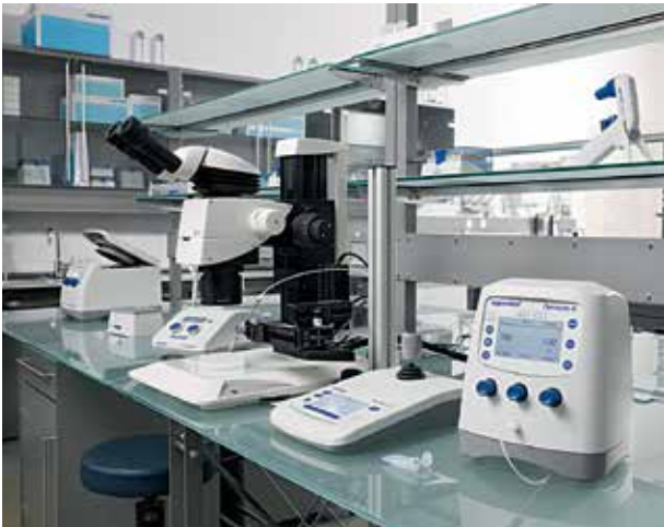
Workstation for injection into fish embryos - InjectMan 4 and FemtoJet setup next to Olympus® SZX16
